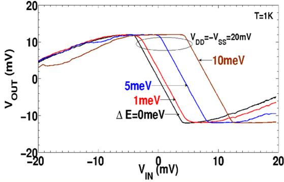
Fig. 3. Influence of energy quantization  $\Delta E$  on  $V_{OUT}$  versus  $V_{IN}$  characteristics at constant  $V_{DD} = -V_{SS} = 20$  mV plotted for capacitance ratio  $\alpha = C_T/C_G = 1/3$  (simulated for  $R_T = 1$  M $\Omega$  and  $C_G + C_T = 4$  aF).
