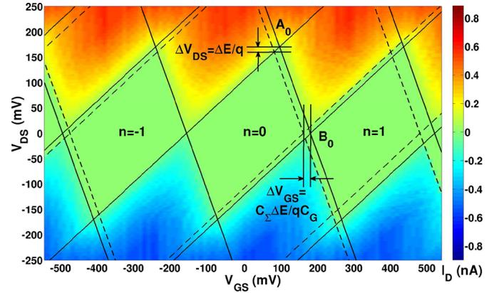
Fig. 2. Influence of energy quantization on  $V_{DS} - V_{GS}$  surface characteristics (drain current contour) of an SET. The solid and broken lines represent the solution of  $\Delta F = 0$  for quantized ( $\Delta E = 10 \text{ meV}$ ) and continuous ( $\Delta E = 0$ ) energy levels in the island, respectively. (simulated for  $R_T = 1 \text{ M}\Omega$ ,  $C_G = 0.5 \text{ aF}$ ,  $C_T = 0.25 \text{ aF}$ , and temperature  $T < q^2/k_B C_\Sigma = 90 \text{ K}$ ).
