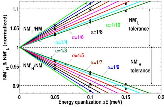
Fig. 6. Variation of normalized noise margins  $NM'_H/NM$  and  $NM'_L/NM$  of the SET inverter with energy quantization  $\Delta E$  for different  $\alpha = C_T/C_G$  ratios at constant  $V_{DD} = 20$  mV bias. The symbols represent simulated data while solid lines indicate the results predicted by the model (noise margin tolerance is taken as 10% of the orthodox value).
