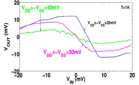
Fig. 4. Influence of bias  $V_{DD} (= -V_{SS})$  on  $V_{OUT}$  versus  $V_{IN}$  characteristics at constant  $\Delta E = 5$  meV plotted for capacitance ratio  $\alpha = C_T/C_G = 1/3$  (simulated for  $R_T = 1$  M $\Omega$  and  $C_G + C_T = 4$  aF).
