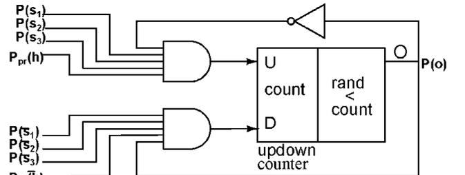
Fig. 3. Neuron circuit in the SBN model. The circuit performs the inference of the external hidden variable using the odd of the likelihood ratio computed by the synapse circuits, and the prior probability of hidden variable.
