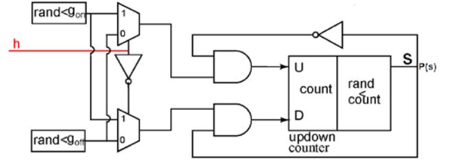
Fig. 2. Synapse circuit in the SBN model. The circuit generates spike trains based on its internal parameters  $g_{on}$  and  $g_{off}$  as the evidence of the external hidden variable.
