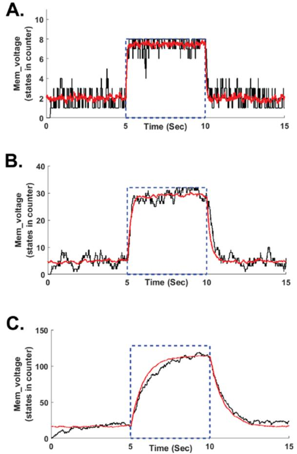
Fig. 5. Evolution of membrane voltage for different time constants, i.e., different counter bit-widths, (A) 3-bit, (B) 5-bit, (C) 7-bit. The blue square indicates the presence of the hidden variable. The red and black curves show the mean membrane voltage across 20 trials and 1 trial, respectively.
