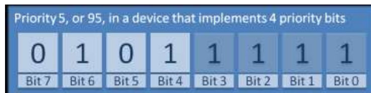
Figure 62 How a priority of binary 101 is stored by a Cortex-M microcontroller that implements four priority bits
