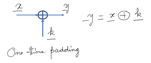
FIGURE 1. Vernam cipher for generating encrypted data.
