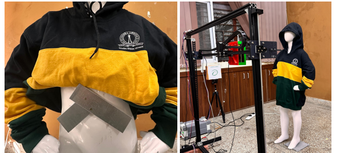
Fig. 4. Concealed weapon detection: the optical image of the scene under radar illumination in our experimental setup.
