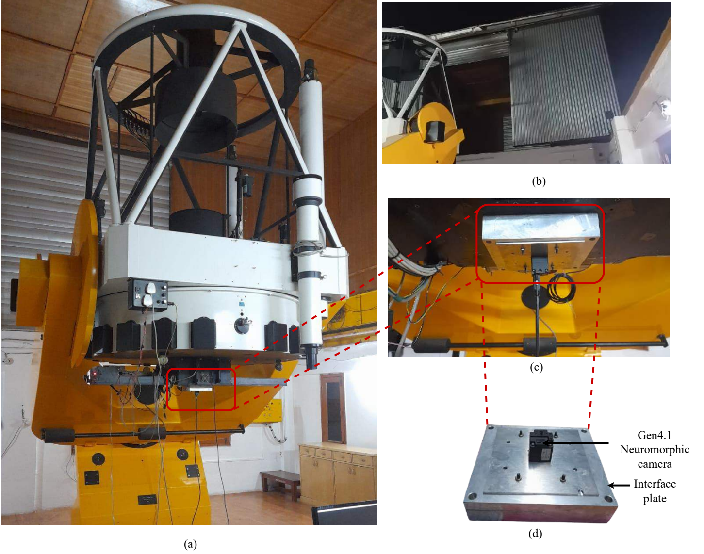
Fig. 3 Observational setup for neuromorphic camera-based celestial observations using the 1300 mm DFOT telescope at Devasthal, ARIES, India. (a) The neuromorphic camera installed at the focal plane of the telescope. (b) Roll-off rooftop moving back to expose the telescope to the night sky. (c) Close-up view of the neuromorphic camera mounted on telescope using a custom interface plate. (d) The neuromorphic camera integrated with the interface plate.
