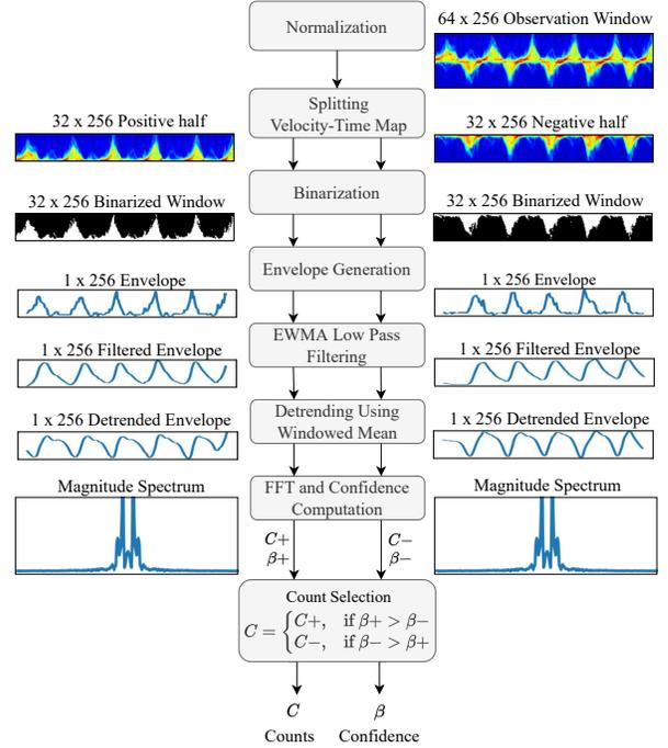
Fig. 5. Repetition counts algorithm flowchart showing each step and the corresponding output.
