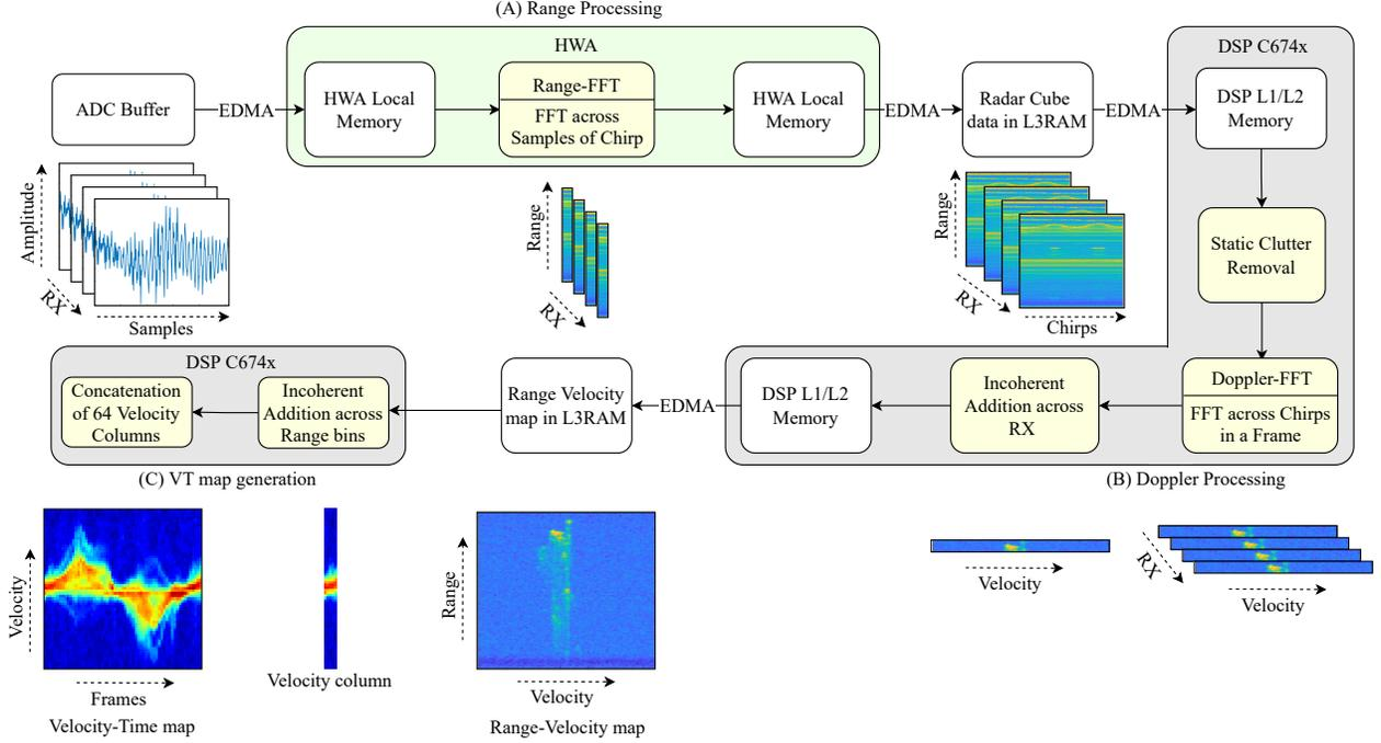
Fig. 3. Flow chart showing radar signal processing steps, the intermediate outputs, and the data flow among different cores of radar board for generation of the VT map. The white blocks symbolize the different memory elements of the radar board. (A) Range processing on the ADC samples of a single chirp for all the RX at a time. (B) Doppler processing on the chirps of a single range bin for all the RX at a time. (C) Velocity-Time map generation.
