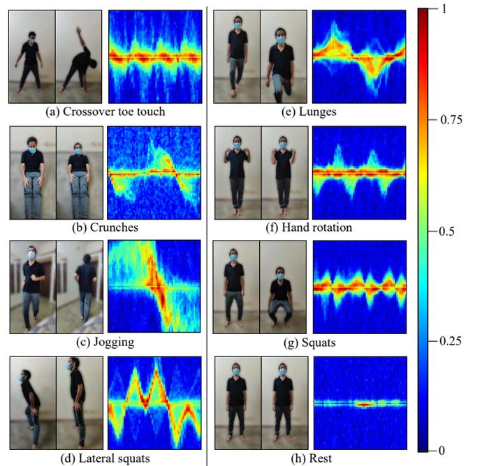
Fig. 2. Exercise types and their VT maps: Snapshots of exercise performed by the user (left) and corresponding normalized VT map (right). In VT maps, the x-axis represents time ranging from 0 to 4.5 seconds, and the y-axis represents velocity ranging from  $-2$  to  $+2$  m/s.
