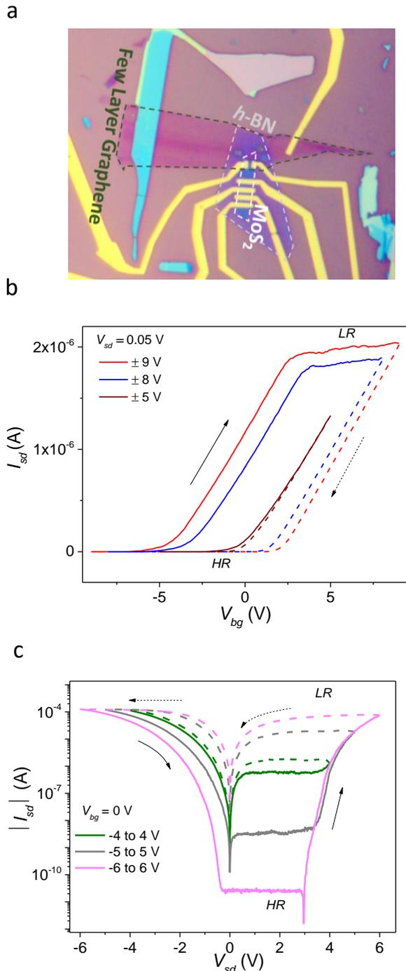
FIG. 2: **Electrical characterization of MoS<sub>2</sub> FG-FET.** **a**, Optical micrograph of a typical MoS<sub>2</sub> FG-FET with individual layers outlined. **b**, and **c**, show the transfer and output characteristics, respectively, for MoS<sub>2</sub> FG-FET. Solid lines denote forward sweep directions (from -ve to +ve values) and dashed lines reverse sweep directions (from +ve to -ve values) in both graphs.
