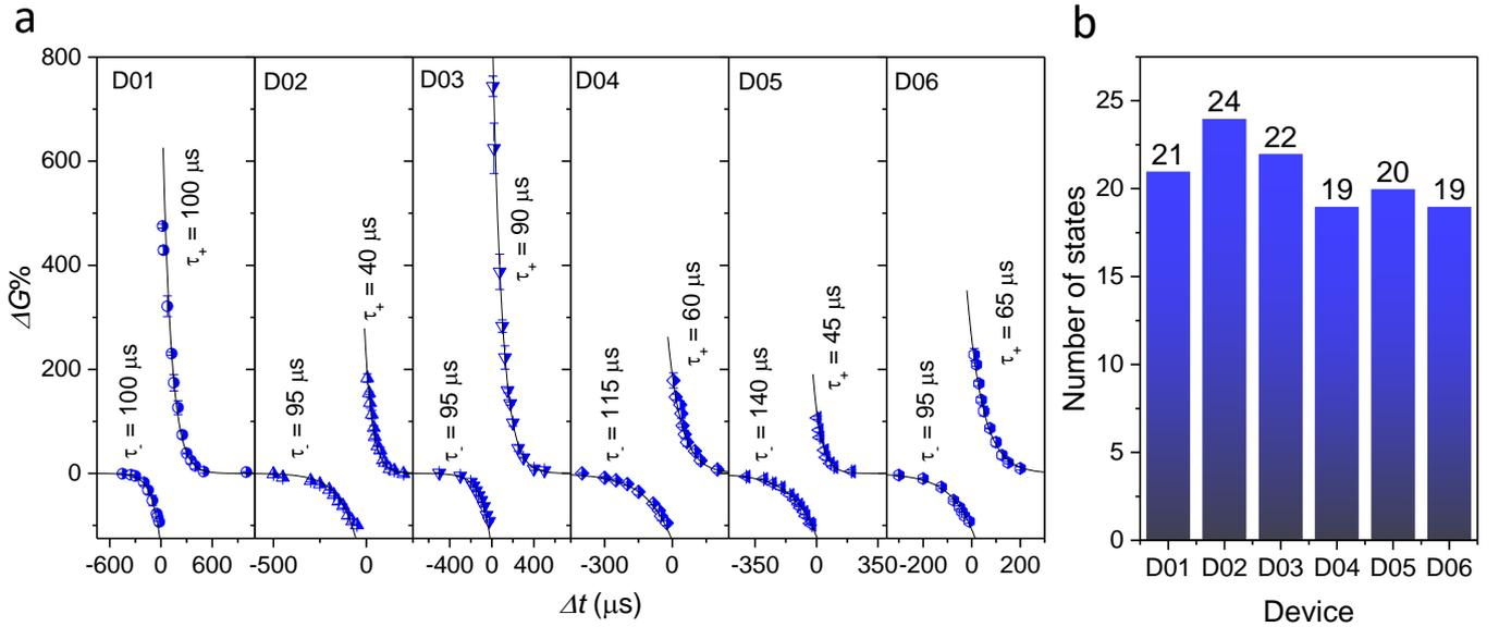
FIG. 6: **Device-to-device variation in STDP response.** **a**, Plots of STDP response for six MoS<sub>2</sub> FG-FETs. Black lines are exponential fits to the experimental data for measuring the decay timescale, while error bars indicate the spread of each state in the  $\Delta G\%$  axis. **b**, Comparison of the number of states in different devices.
